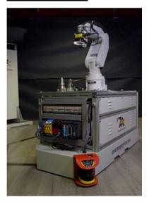
**Photo 1:** The AGV can move around the assembly line following a path traced by magnetic tape and is equipped with safety scanners that allow the device to stop if an obstacle is found en route.
