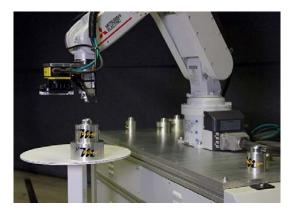
**Photo 3:** The AGV-mounted robot can move along a production line and perform jobs such as product assembly, pick-and-place or packaging tasks.
