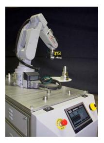
**Photo 2:** Operators can interact with the robot and AGV via a Mitsubishi Electric graphic operator terminal (GOT) or remotely, using a Wi-Fi connected master control box.
